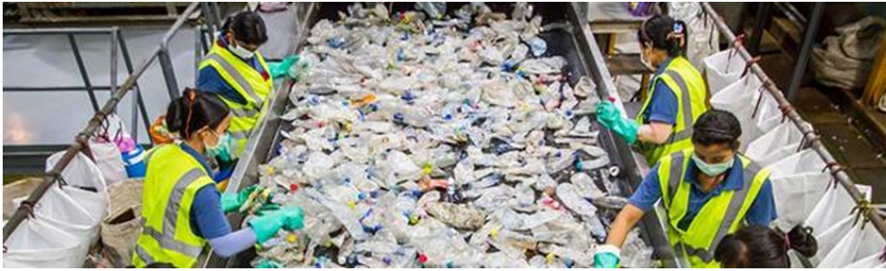
Figure 4 Sorting process of PET bottle wastes [12]
